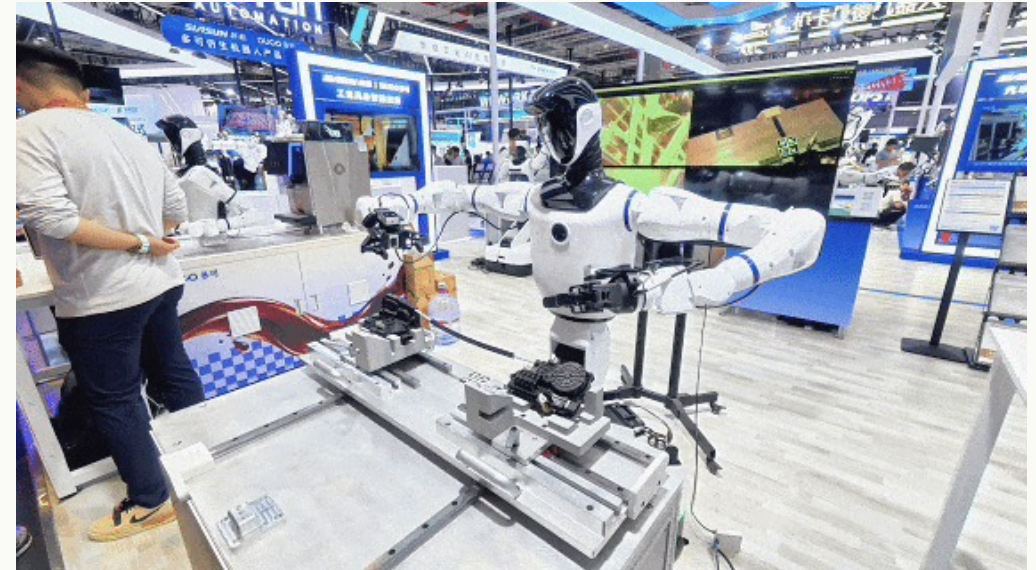
SIASUN BR-MR73A car-lock inspection
